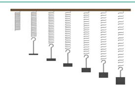
Students placed masses, one at a time, on a spring and measured its extension. They collected the following results.
